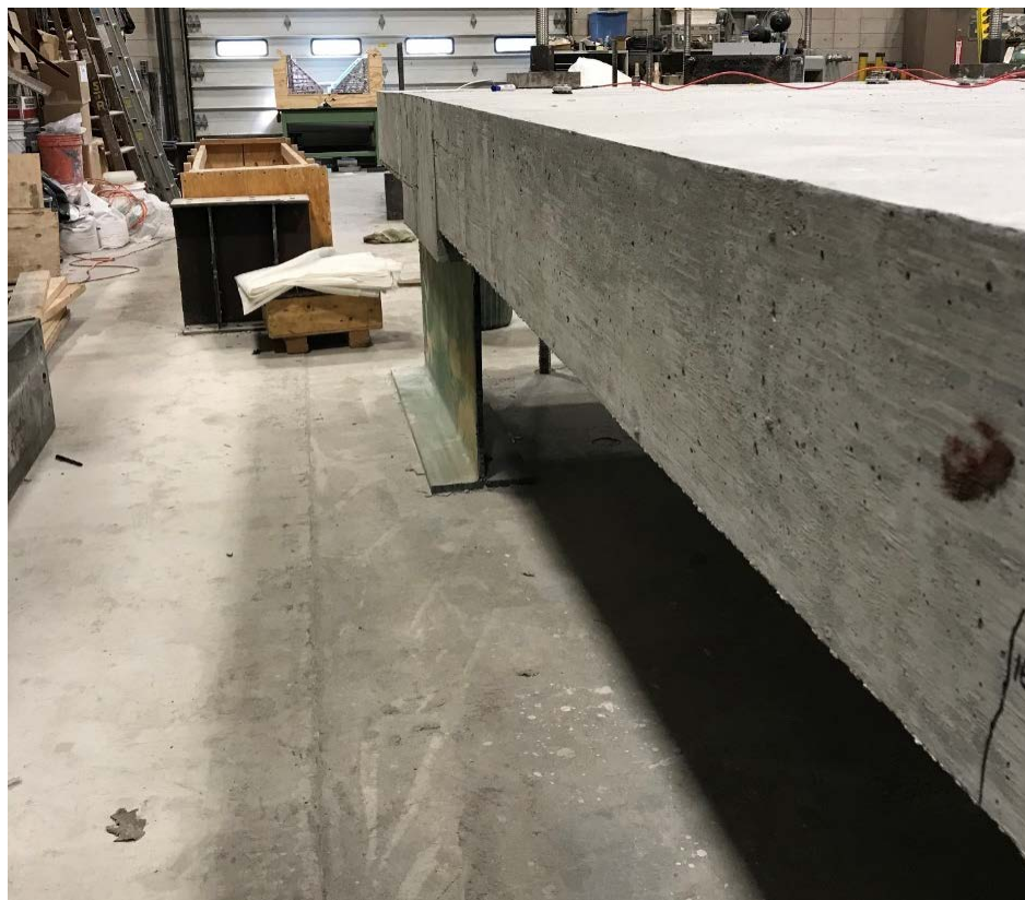
Figure 2-43. Side view of deflection of lab specimen and rotation at beginning of approach slab, Test 2.
