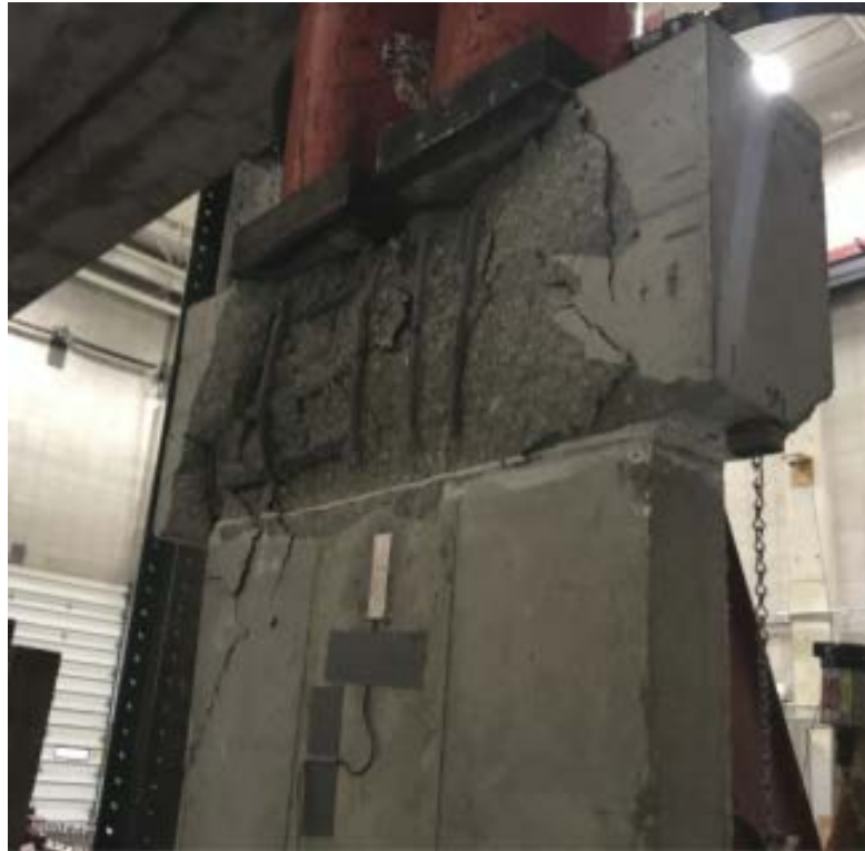
Figure 3-8. Bursting of top reinforced concrete block.
