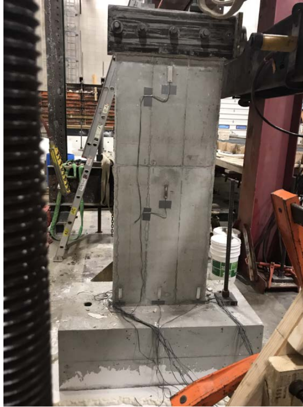
Figure 3-24. Pushover test setup.
