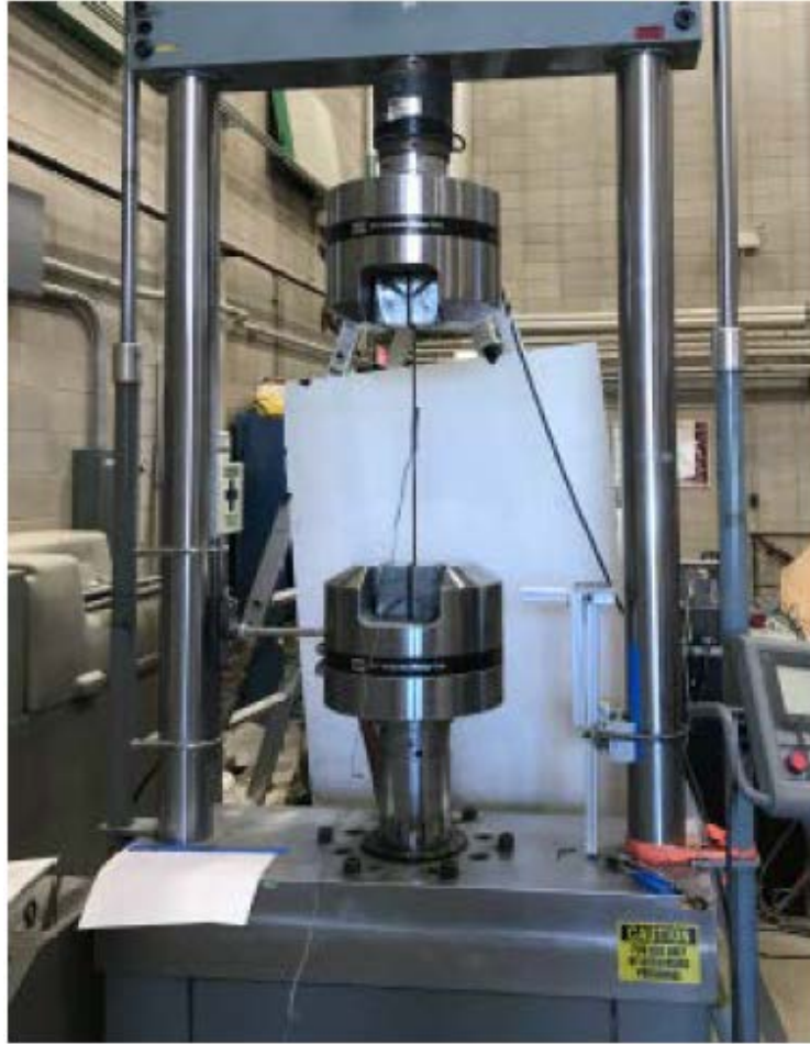
Figure 3-5. Uniaxial testing of NO. 2 reinforcing bar.
