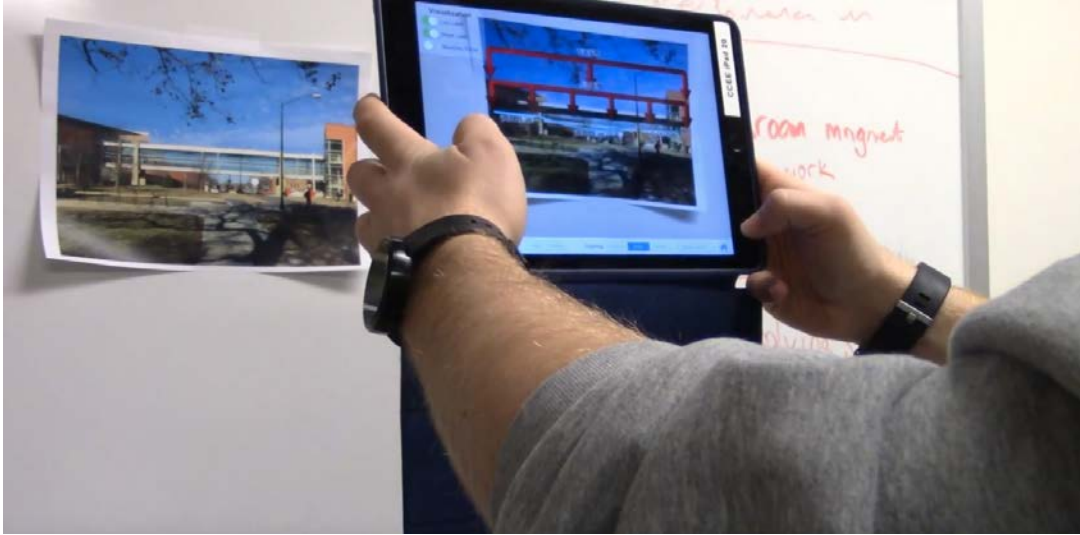
Figure 4-9. Student changes the magnitude and location of the live load on a printed photo of the skywalk through augmentation.
