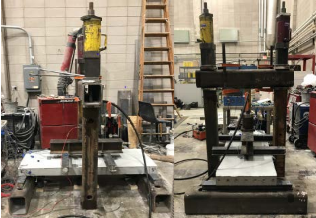
Figure 3-16. Testing setup for four-point bending test.
