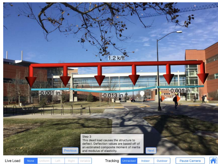
Figure 4-3. Guided version of skywalk application, with an example procedural step explaining deflection values.
