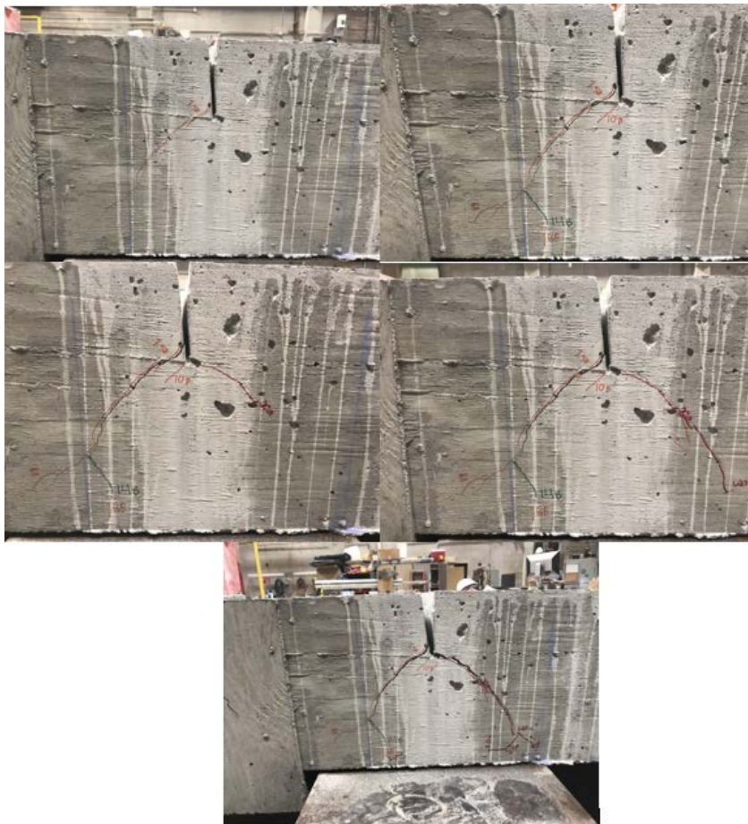
Figure 2-38. Crushing occurring at midspan of approach slab at failure, Test 2.
