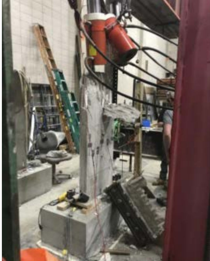
Figure 3-10. Failure of second axial load test wall.
