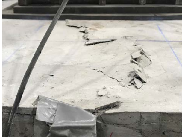
Figure 2-38. Crushing occurring at midspan of approach slab at failure, Test 2.
