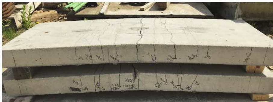
Figure 3-21. Cracking on sides of walls, four-point bending test.
