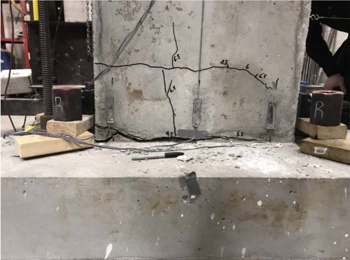
Figure 3-25. Cracking at bottom of wall, pushover test.
