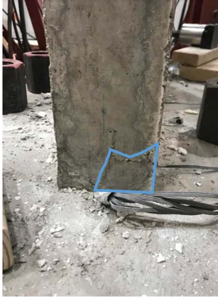
Figure 3-65. Area of minimal crushing in laboratory specimen, pushover test.
