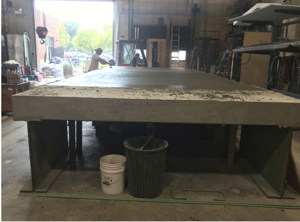
Figure 2-15. Laboratory specimen when approach slab and diaphragm sections are poured; view of steel girders.
