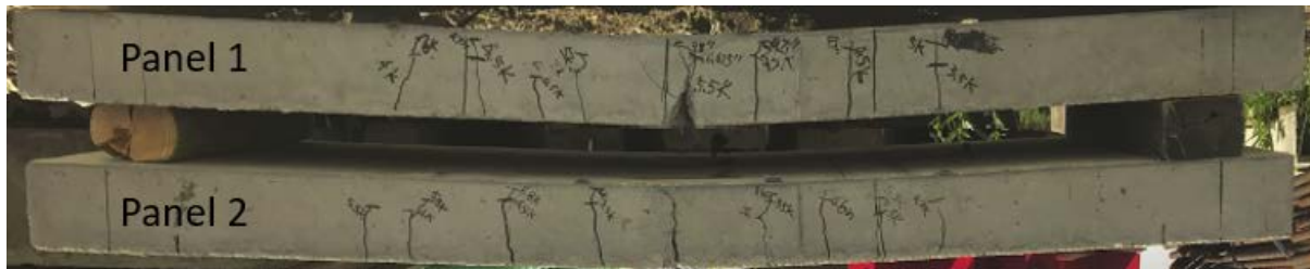
Figure 3-21. Cracking on sides of walls, four-point bending test.
