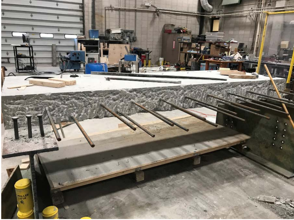
Figure 2-13. Construction joint at interface of existing bridge deck and concrete diaphragm sections.
